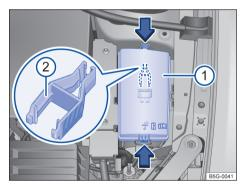
**Fig. 158** In the engine compartment: fuse box cover ① with plastic claw ②.
