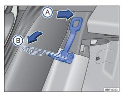
Fig. 64 Behind the rear seat: seat backrest rake adiustment lever
