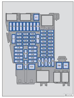
Fig. 157 On the dash panel: fuses arrangement.
