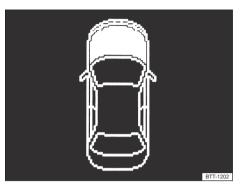
**Fig. 169** On the instrument cluster display: incorrectly closed or open bonnet (schematic representation).
