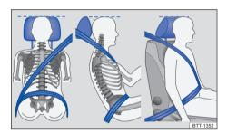
**Fig. 29** Correct seat belt routing and head rest adjustment.
