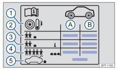
Fig. 179 Sticker with the tyre pressures.
