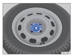
Fig. 182 On the luggage compartment: spare wheel fastening handwheel.
