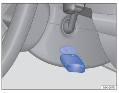
**Fig. 92** To the right of the steering column: emergency start function of vehicles with Keyless Access locking and start system.
