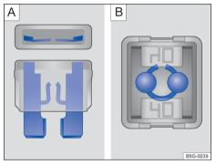
Fig. 161 Blown fuse: A flat fuse, B blocking fuse.
