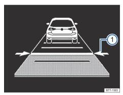
Fig. 111 On the instrument cluster display: adjust the distance (schematic view, the ACC will adjust).
