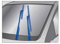
Fig. 153 Window wipers in service position.
