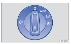
**Fig. 71** Next to the steering wheel: light switch (one variant).
