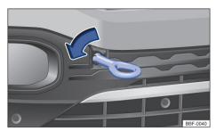
**Fig. 166** On the right-hand side of the front bumper: screw in the towing eye.
