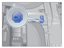
**Fig. 163** On the engine compartment: jump starting point (grounding point).
