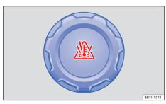
**Fig. 174** On the engine compartment: engine coolant expansion tank cover.
