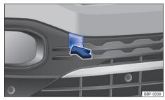
**Fig. 165** On the right-hand side of the front bumper: release and remove the cover.
