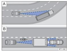
Fig. 108 A Curve condition. B Vehicles outside the radar sensor range
