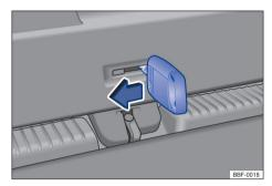
Fig. 58 In the luggage compartment: unlock the boot lid.
