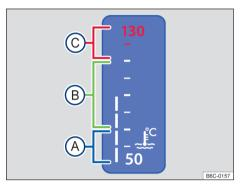
**Fig. 13** Engine coolant temperature indicator in the digital instrument cluster (version 1): (a) cold zone; (b) normal zone; (c) warning zone.
