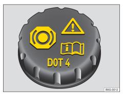
Fig. 175 On the engine compartment: brake fluid reservoir cap.
