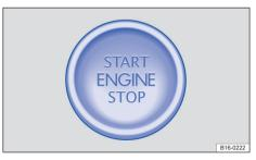
**Fig. 91** On the lower part of the centre console: engine start button.
