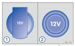
Fig. 131 12-V socket with folding cover ①, 12-V with removable cover ②.
