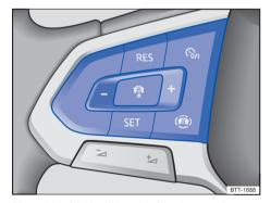
**Fig. 110** Left side of the multifunction steering wheel: ACC operating buttons.
