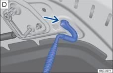
Fig. 168 C Bonnet stay. D Bonnet secured with the bonnet stay.
