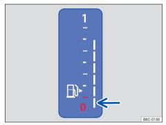
Fig. 11 On the digital instrument cluster: fuel gauge (version 1).
