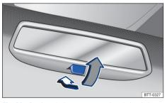
**Fig. 80** On the windscreen: manual anti-dazzle interior mirror.
