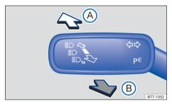
Fig. 72 On the left on the steering column: turn signal and main beam lever.
