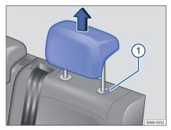
Fig. 68 Rear seat head restraint: removal
