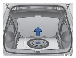
**Fig. 150** On the luggage compartment, under the floor lining: spare wheel and vehicle toolkit.
