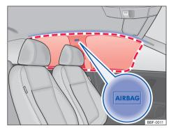
**Fig. 38** Left side of the vehicle: location and deployment zone of the curtain airbag.
