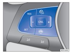
Fig. 105 Left side of the multifunction steering wheel (version 1): speed limiter operating buttons.
