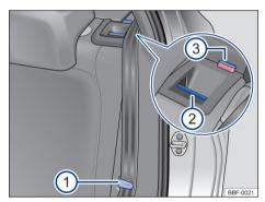
Fig. 63 On the rear seat backrest: unlocking button.
