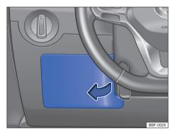
**Fig. 156** On the driver's side of the dashboard: fuse box cover.
