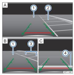
Fig. 117 Exhibition on the radio system display: parking with the rear view camera system.
