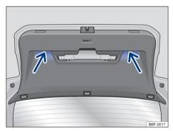
Fig. 57 Open boot lid: recesses (arrows) to pull and close.
