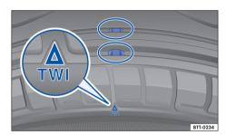
Fig. 181 Tyre profile: wear indicators.
