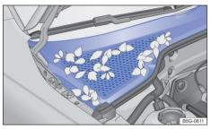
**Fig. 189** Between the engine compartment and the windscreen: plenum chamber (schematic representation).
