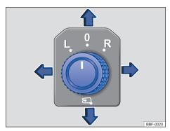
Fig. 81 On the driver door: rotary adjusting knob for the electric exterior mirrors.
