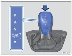
**Fig. 96** Automatic gearbox selector lever with interlock button (arrow).
