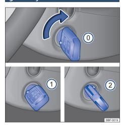
**Fig. 90** Next to the steering wheel, to the right: vehicle key positions on the ignition cylinder.
