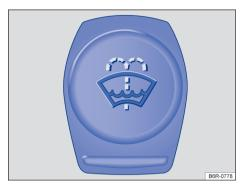
**Fig. 170** On the engine compartment: window washer fluid reservoir cap.
