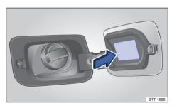
Fig. 180 On the inner side of the fuel tank flap: tyre pressure label.
