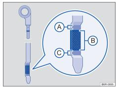
Fig. 171 Oil dipstick with markings.
