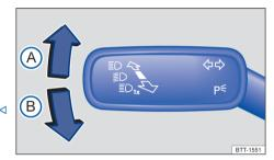
**Fig. 73** On the left on the steering column: turn signal and main beam lever.
