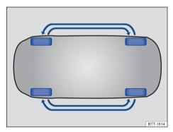
Fig. 178 Diagram showing how to swap wheels.
