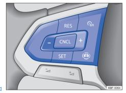
Fig. 106 Left side of the multifunction steering wheel (version 2): speed limiter operating buttons.
