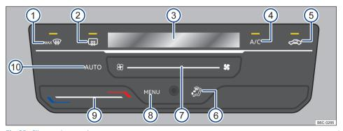
Fig. 85 Climatronic controls.
