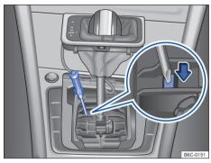
**Fig. 99** Remove the selector lever cover and manually emergency unlock the selector lever lock.
