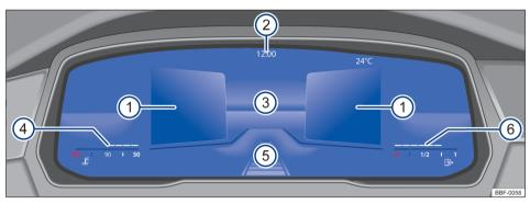
Fig. 10 Active Info Display on the dash panel (version 2).
