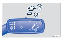
**Fig. 77** To the right of the steering column: control the rear window wiper/washer.
