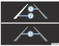
**Fig. 112** On the instrument cluster: lane keeping assistant display indicators.
