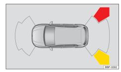
Fig. 123 Infotainment system: display of the Rear Traffic Alert
