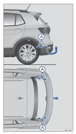
**Fig. 148** Attachment points for retrofitting a towing bracket.
