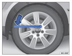
Fig. 184 Changing the wheel: loosen wheel bolts.
