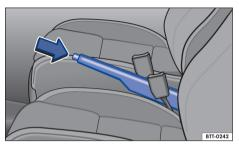
Fig. 114 Between front seats: handbrake lever.
