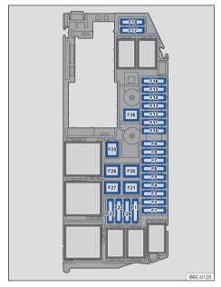
**Fig. 159** In the engine compartment: fuse arrangement.
