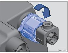
**Fig. 75** In the engine compartment: headlight range control switch (variant 2).
