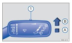
Fig. 78 To the right of the steering column: window wipers lever.
