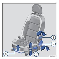
Fig. 62 On the front seat: controls.
