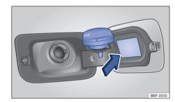
Fig. 149 Open tank flap with tank cap attached to the holder.
