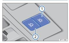
Fig. 83 On the headliner: sun blind control buttons.
