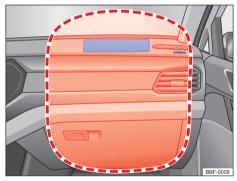
**Fig. 34** Installation location and expansion zone of the passenger front airbag.
