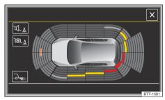
**Fig. 116** Indication on the radio system: full screen mode. The detected areas depend on the vehicle version.
