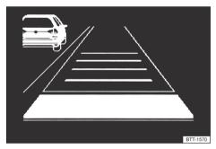
**Fig. 107** On the instrument cluster display: slower vehicle detected on the left-hand lane (schematic view).
