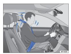
**Fig. 26** Driver restrained by a properly positioned seat belt during a sudden braking manoeuvre.
