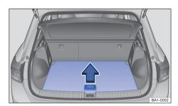
**Fig. 145** In the luggage compartment: raise the luggage compartment floor.
