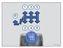
**Fig. 95** Gear shift pattern of a 6-speed manual gearbox.
