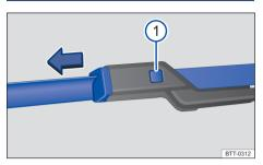
Fig. 154 Replacing windscreen wiper blades.
