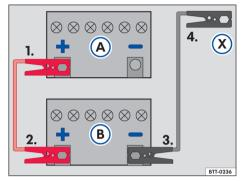
**Fig. 164** Jump lead attachment diagram: discharged vehicle battery (A) and battery in the vehicle providing assistance (B).
