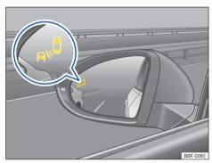
**Fig. 113** On the exterior mirrors: Blind Spot Monitor indicator.
