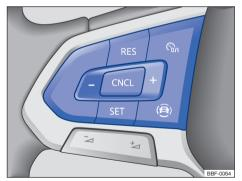
**Fig. 104** Left side of the multifunction steering wheel (version 2): GRA operating buttons.
