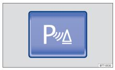
**Fig. 115** On the centre console: manual park distance control on/off button.
