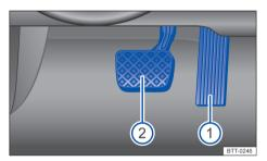
**Fig. 87** In the footwell: pedals in vehicles with automatic gearbox.
