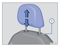
Fig. 65 Front seat head restraint: adjust.
