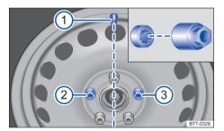
**Fig. 185** Wheel change: Tyre valve ① and installation position of the anti-theft wheel bolt ② or ③.
