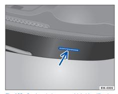
**Fig. 193** On the windscreen: vehicle identification number.
