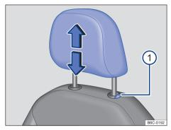
Fig. 67 Front seat head restraint: removal.
