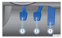
**Fig. 86** In the footwell: pedals in vehicles with manual transmission.
