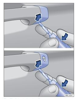
Fig. 53 Driver's door handle: remove cover.
