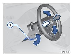
**Fig. 60** Below and to the left of the steering wheel next to the steering column trim: steering wheel position adjustment lever.
