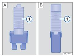
**Fig. 162** Removing or installing the fuse with the plastic claw: A: flat fuse, B blocking fuse.
