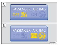
Fig. 32 In the upper part of the centre console: front passenger front airbag indicator lamp off A or on B.
