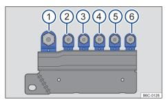
**Fig. 160** In the engine compartment on top of the battery: fuse arrangement.
