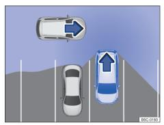
**Fig. 122** Monitored area around the vehicle that will leave the parking space (schematic representation).
