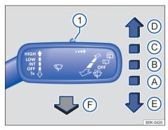
**Fig. 76** To the right of the steering column: control the windscreen wipers/washers.
