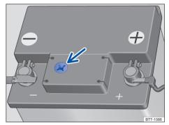
**Fig. 176** On the engine compartment: example of display position on the upper side of the vehicle battery.
