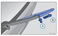
Fig. 155 Replacing the rear window wiper blades.
