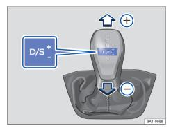
Fig. 97 Selector lever in Tiptronic position.
