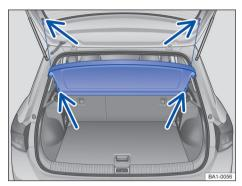
**Fig. 144** In the luggage compartment: remove and install the luggage compartment cover.
