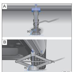
Fig. 187 Jacking points and vehicle jack at the rear left-hand side of the vehicle.
