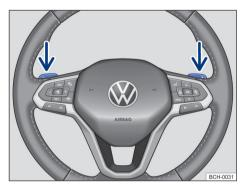
**Fig. 98** Steering wheel with Tiptronic gear shift paddles.
