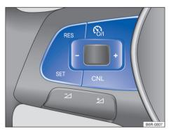
Fig. 103 Left side of the multifunction steering wheel (version 1): GRA operating buttons.
