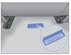
**Fig. 192** In front of the rear passenger seat, on the right-hand side of the floor: vehicle identification number (running gear number).
