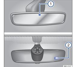
**Fig. 79** On the windscreen: automatic anti-dazzle interior mirror.
