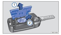
Fig. 48 Vehicle key: replacing the battery.
