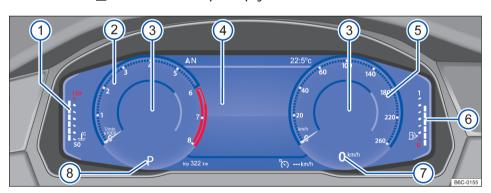
Fig. 9 Active Info Display on the dash panel (version 1).
