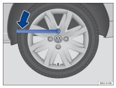
Fig. 170 Changing the wheel: loosen wheel bolts.
