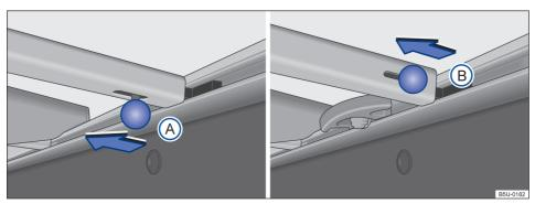
**Fig. 50** Luggage compartment cross struts: (A) vehicles with fixed strapping supports, (B) vehicles with sliding strapping supports.
