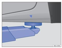
**Fig. 175** Rear lifting points for lifting with platform or vehicle jack.
