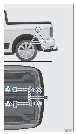
Fig. 124 Attachment points for retrofitting a towing bracket.
