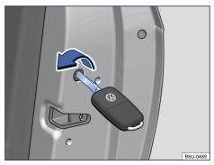
**Fig. 45** Emergency vehicle locking with the vehicle key.
