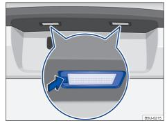
**Fig. 139** On the rear bumper: remove the number plate light.
