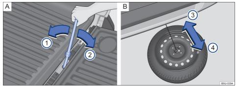
**Fig. 165** A In the cargo compartment: access to the temporary spare wheel. B Under the vehicle: spare wheel entirely on the floor and removal from underneath the vehicle.
