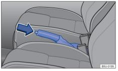
Fig. 88 Between front seats: handbrake lever.
