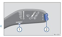
**Fig. 17** Vehicles without multifunction steering wheel: press button ① in the windscreen wiper lever to confirm the menu point and rocker switch ② to switch between menus.
