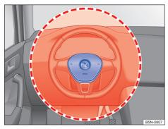
Fig. 33 Location and deployment zone of the driver front airbag.
