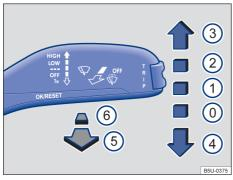
Fig. 67 Windscreen wiper / washer controls.
