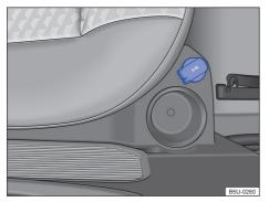
**Fig. 107** On the side of the rear seat: 12-volt socket - New Saveiro with extended cab.
