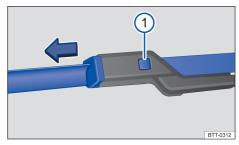
Fig. 133 Replacing windscreen wiper blades.
