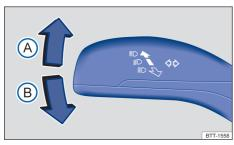
**Fig. 60** On the left on the steering column: turn signal and main beam lever.
