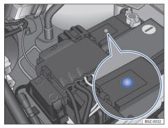
**Fig. 159** On the engine compartment: example of display position on the upper side of the vehicle battery.
