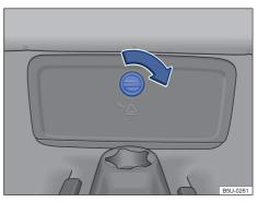
Fig. 128 On the rear seat floor: access to the vehicle toolkit housing.
