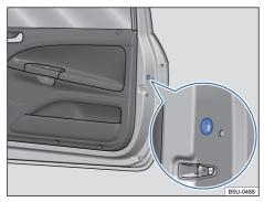
**Fig. 44** Front part of the right-hand door: emergency vehicle locking, covered by a rubber seal.
