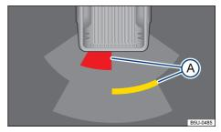
**Fig. 90** Parking distance control display (coloured display): (A) obstacle identified in the segment.
