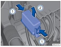
Fig. 145 On the engine compartment: fuse box cover.
