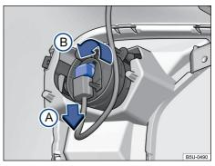
Fig. 137 Behind the front bumper: access to the fog light bulb.
