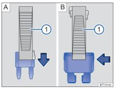
**Fig. 148** Removing or fitting a fuse using the plastic pliers ①.
