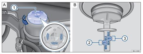
**Fig. 85** On the engine compartment: A Power steering fluid reservoir. B Power steering fluid level control marks.
