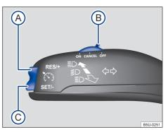
**Fig. 87** To the left on the steering column: lever with switch and GRA operating buttons.
