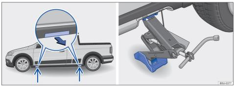
Fig. 172 Jacking points and vehicle jack at the rear left-hand side of the vehicle - vehicles with external sills.
