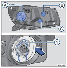
**Fig. 135** In the engine compartment: rear view of the headlight with rubber cover (left side of illustration) - (A) dipped beam / main beam, (B) B daytime running light / side light and (C) turn signals. Rear view of the front headlight without the rubber cover (right-hand side of the illustration): (1) locking spring of the dipped beam / main beam headlight bulb.
