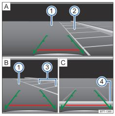
**Fig. 92** Display of the radio or navigation system: enter the parking spot with the rear view camera (schematic display).
