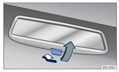
Fig. 69 On the windscreen: manual anti-dazzle interior mirror.
