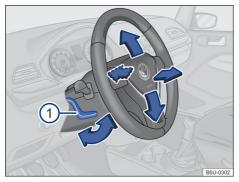
**Fig. 55** Below and to the left of the steering wheel next to the steering column trim: steering wheel position adjustment lever.
