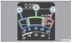
Fig. 14 Engine coolant temperature indicator in the instrument cluster (variable 1): (A) cold zone; (B) normal zone; (C) warning zone.
