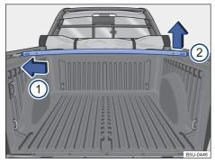
Fig. 52 Bed crossmembers - remove and install.
