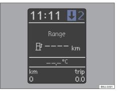
**Fig. 80** On the instrument cluster: gearshift indicator (variable 2).
