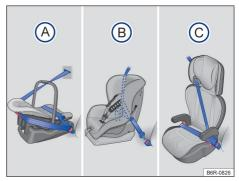
**Fig. 36** Figures (**A**), (**B**) and (**C**) illustrate the main securing points for the child restraint system for children only wearing the seat belt.
