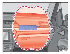
**Fig. 34** Location and deployment zone of the passenger front airbag.
