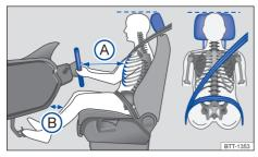
**Fig. 20** Correct distance between the driver and the steering wheel, correct seatbelt position and correct headrest adjustment.
