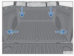
Fig. 118 Bed: strapping eyelets.
