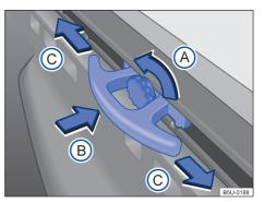
**Fig. 121** On the bed: sliding support for vehicles with bed canvas.
