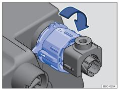
**Fig. 63** In the engine compartment: headlight range adjustment switch.
