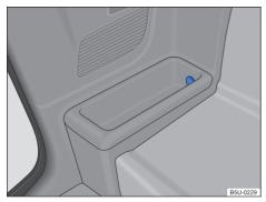
Fig. 105 In the side panel of the internal luggage compartment:12 V socket.
