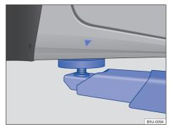
**Fig. 174** Front lifting points for lifting with platform or vehicle jack.
