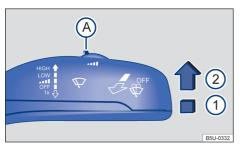
Fig. 68 Windscreen wiper lever: adjust rain sensor sensitivity (A).
