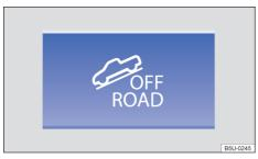
**Fig. 86** On the centre console: manual off-road mode on/off button.
