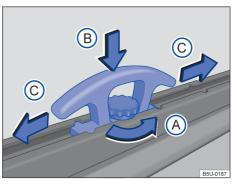
**Fig. 120** On the bed: sliding support for vehicles without bed canvas.
