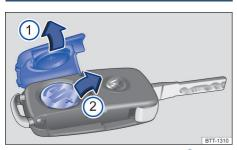
**Fig. 41** Vehicle key with remote control: ① Open the battery case cover. ② Remove the battery.
