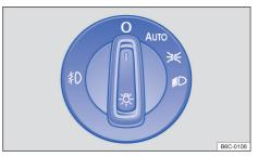
Fig. 61 Next to the steering wheel: light switch.
