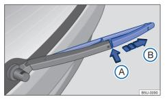
Fig. 132 Replacing the rear window wiper blades.
