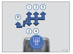
**Fig. 84** Gear shift pattern of a 5-speed manual gearbox.
