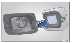
**Fig. 163** On the inner side of the fuel tank flap: tyre pressure label.
