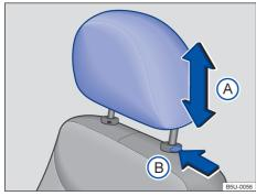
Fig. 58 Front head restraint: adjust, remove and install.
