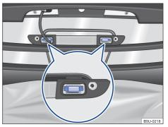
**Fig. 142** Elevated brake light: remove the bulb from the bed light.
