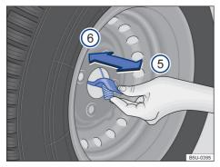
**Fig. 166** On the spare wheel: remove the spare wheel cable.
