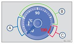
**Fig. 15** Engine coolant temperature indicator in the instrument cluster (variable 2): (A) cold zone; (B) normal zone; (C) warning zone.
