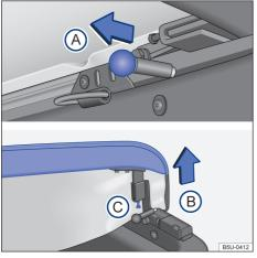
Fig. 48 Bed canvas stretching adjustment locks and bolt.
