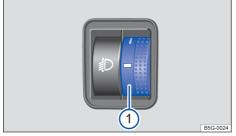
Fig. 64 Next to the steering wheel: control of the headlight range 1
