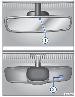
Fig. 70 On the windscreen: automatic anti-dazzle interior mirror.
