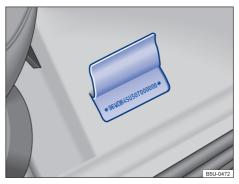
**Fig. 177** In front of the front passenger seat: vehicle identification number (chassis number) on the floor, in front of the passenger seat.
