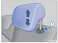
Fig. 59 Rear head restraint: adjust, remove and install.
