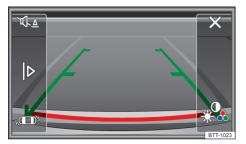
**Fig. 91** Display of the radio or navigation system: reverse camera turned on (schematic).
