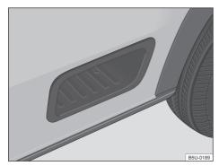
Fig. 122 On the vehicle's side: bed access step.
