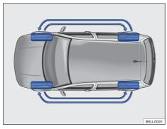
Fig. 161 Diagram showing how to swap wheels.
