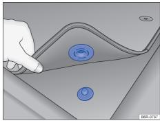
Fig. 19 Driver side mat attached to the floor pin.
