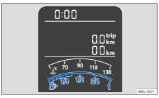
**Fig. 12** On the instrument cluster display: fuel gauge (variable 1).
