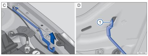
Fig. 152 C Bonnet stay. D Bonnet secured with the bonnet stay.
