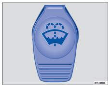
**Fig. 153** On the engine compartment: windscreen washer fluid reservoir cap.
