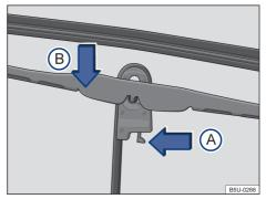
Fig. 131 Replacing windscreen wiper blades.
