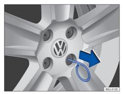
Fig. 168 Removing the wheel bolt caps.
