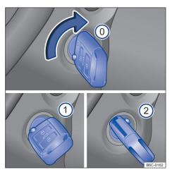
**Fig. 82** Next to the steering wheel, to the right: vehicle key positions on the ignition cylinder.
