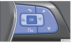
**Fig. 18** Right-hand side of the multifunction steering wheel: instrument cluster menu control buttons.
