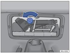
Fig. 129 Vehicle toolkit fastening handle.
