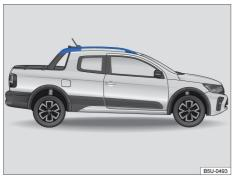
**Fig. 123** Roof rack longitudinal supports (both sides).
