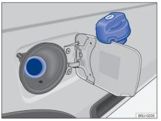
**Fig. 125** Open tank flap with tank cap attached to the holder.
