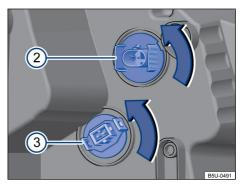
**Fig. 136** In the engine compartment: rear view of the front headlight (2) daytime running light / side light and (3) turn signals.
