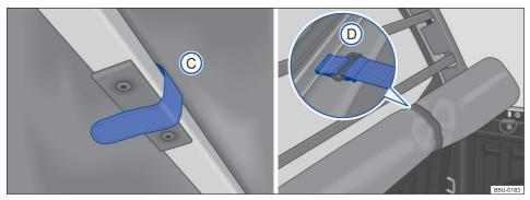
Fig. 51 On the bed: fastening strap and bed canvas properly retracted.
