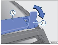
Fig. 117 On the roof: cross member and pivot support.
