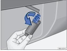
Fig. 140 Number plate light: remove the bulb socket.
