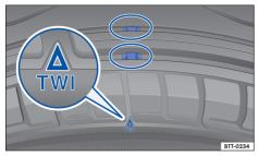
Fig. 164 Tyre profile: wear indicators.
