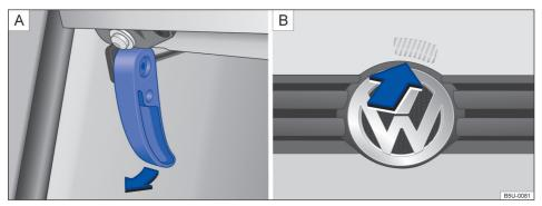
Fig. 151 A Bonnet release lever on the driver side footwell. B Bonnet release lever on the inner side of the bonnet.
