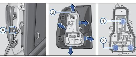
Fig. 138 Tail light: (C) remove the bulb support and (1), (2), (3), (4) e (5) remove the bulbs.
