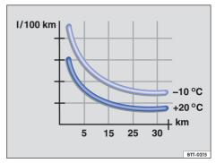
**Fig. 81** Fuel consumption in litres per 100 km at two distinct ambient temperatures.
