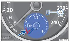
Fig. 13 On the instrument cluster: fuel gauge (variable 2).
