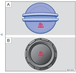
**Fig. 157** On the engine compartment: A cap of the engine coolant expansion reservoir (variant 1) or B cap of the engine coolant expansion reservoir (variant 2)
