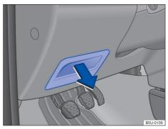
**Fig. 143** On the driver's side of the dashboard: fuse box cover.
