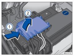
Fig. 149 Engine compartment: access to the positive battery terminal.
