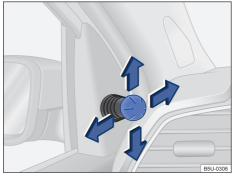
Fig. 71 On the front doors: setting knob for the mechanical exterior mirrors.
