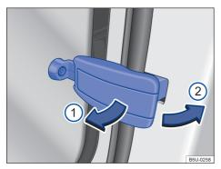
Fig. 54 Close the rear vent window.
