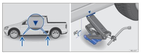
Fig. 171 Jacking points and vehicle jack at the rear left-hand side of the vehicle.
