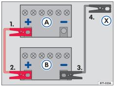
**Fig. 150** Jump lead attachment diagram: discharged vehicle battery (A) and battery in the vehicle providing assistance (B).
