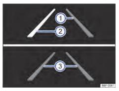
**Fig. 106** On the instrument cluster: lane keeping assistant display indicators.
