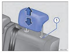
Fig. 64 Rear seat head restraints: adjust.
