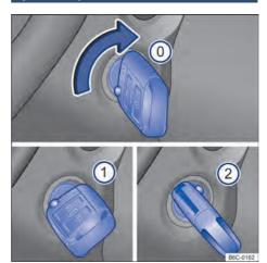
**Fig. 86** Next to the steering wheel, to the right: vehicle key positions on the ignition cylinder.
