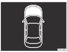
**Fig. 189** On the instrument cluster display: incorrectly closed or open bonnet (schematic representation).
