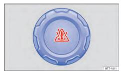
**Fig. 194** On the engine compartment: engine coolant expansion tank cover.
