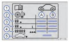
Fig. 199 Sticker with the tyre pressures.
