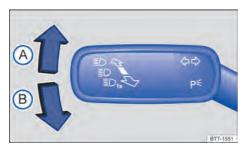
**Fig. 68** On the left on the steering column: turn signal and main beam lever.
