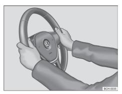
**Fig. 60** On the steering wheel: 9 o'clock and 3 o'clock positions.
