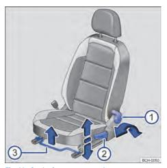
Fig. 61 On the front seat: controls.
