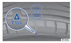
Fig. 201 Tyre profile: wear indicators.
