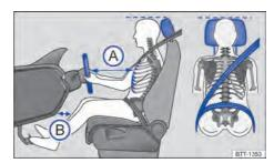
**Fig. 19** Correct distance between the driver and the steering wheel, correct seatbelt position and correct headrest adjustment.
