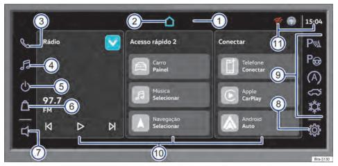
Fig. 154 Overview of controls (variant 2)
