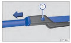
Fig. 174 Replacing windscreen wiper blades.
