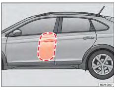
**Fig. 36** On the left side of the vehicle: side airbag deployment zone.
