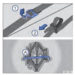
**Fig. 171** On the luggage compartment: vehicle toolkit securing strap and vehicle toolkit.
