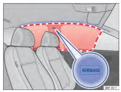
**Fig. 38** Left side of the vehicle: location and deployment zone of the curtain airbag.
