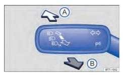
**Fig. 70** On the left on the steering column: turn signal and main beam lever.
