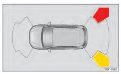
Fig. 118 Infotainment system: display of the Rear Traffic Alert
