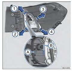
Fig. 177 Tail light: remove the bulb support
