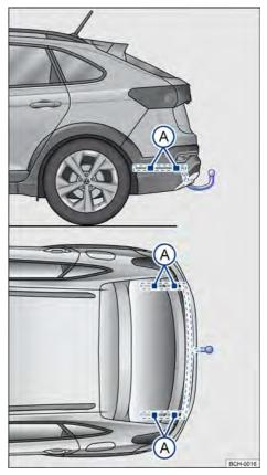
**Fig. 168** Attachment points for retrofitting a towing bracket.
