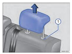
Fig. 66 Rear seat head restraint: removal
