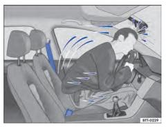
Fig. 24 An unbelted driver is thrown forward.
