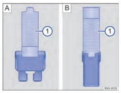
**Fig. 184** Removing or installing the fuse with the plastic claw: A: flat fuse, B blocking fuse.
