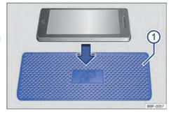
**Fig. 120** Stowage compartment with pad for wireless charging function. The symbol on the lining pad may appear differently in some vehicles.
