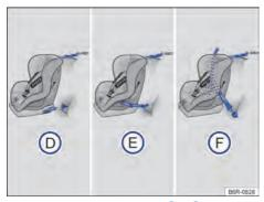
Fig. 40 On the rear seat: figures ( e ( illustrate the securing principle of the child retention system to the bottom retention eyes and the top tether. Figure ( illustrates how to fasten the child restraint system with the vehicle seat belt and the top tether.
