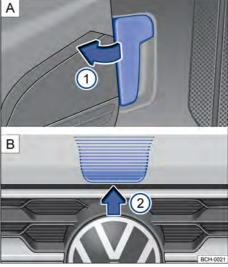
Fig. 187 A Bonnet release lever on the driver side footwell. B Bonnet release lever on the inner side of the bonnet.
