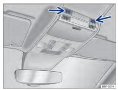
**Fig. 55** On the roof console: vehicle interior monitoring sensors (arrows).
