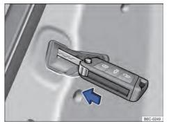
**Fig. 54** On the doors, front right and rear: emergency locking of the vehicle with the metallic stem of the key.
