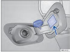
**Fig. 169** Open tank flap with tank cap attached to the holder.
