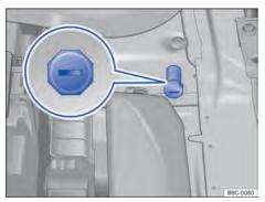
**Fig. 185** On the engine compartment: jump starting point (grounding point).
