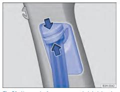
**Fig. 31** Next to the front seats: seat belt height adjuster.
