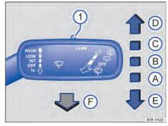
**Fig. 72** To the right of the steering column: control the windscreen wipers/washers.
