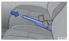
Fig. 110 Between front seats: handbrake lever.
