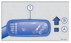
**Fig. 74** To the right of the steering column: window wipers lever.
