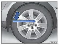
Fig. 204 Changing the wheel: loosen wheel bolts.
