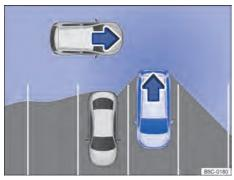
Fig. 117 Monitored area around the vehicle that will leave the parking space (schematic representation).
