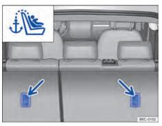
Fig. 42 retention eyes for the top tether on the back side of the rear seat.
