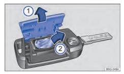
Fig. 48 Vehicle key: replacing the battery.
