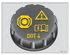
Fig. 195 On the engine compartment: brake fluid reservoir cap.
