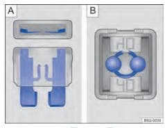
Fig. 183 Blown fuse: A flat fuse, B blocking fuse.
