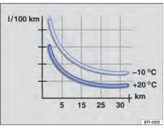
Fig. 85 Fuel consumption in litres per 100 km at two distinct ambient temperatures.
