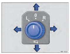
**Fig. 77** On the driver door: rotary adjusting knob for the electric exterior mirrors
