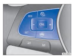
**Fig. 96** Left side of the multifunction steering wheel (version 1): GRA operating buttons.
