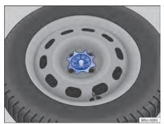
Fig. 202 On the luggage compartment: spare wheel fastening handwheel.
