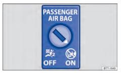
**Fig. 35** On the dash panel on the front passenger side: key activated switch to enable or disable the front passenger front airbag.
