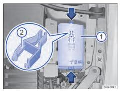
Fig. 180 In the engine compartment: fuse box cover (1) with plastic claw (2).
