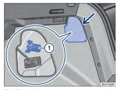
Fig. 176 In the luggage compartment remove the cover and remove the wingbolt ① (magnifying glass)
