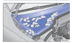
**Fig. 208** Between the engine compartment and the windscreen: plenum chamber (schematic representation).
