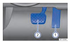
**Fig. 83** In the footwell: pedals in vehicles with automatic gearbox.
