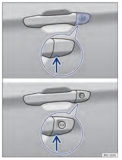
Fig. 52 Driver's door handle: lock cylinder.
