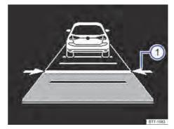
**Fig. 105** On the instrument cluster display: adjust the distance (schematic view, the ACC will adjust).
