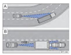
**Fig. 101** A Curve condition. B Vehicles outside the radar sensor range
