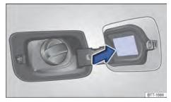
**Fig. 200** On the inner side of the fuel tank flap: tyre pressure label.
