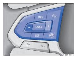
**Fig. 97** Left side of the multifunction steering wheel (version 2): GRA operating buttons.
