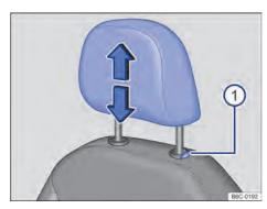
Fig. 65 Front seat head restraint: removal.
