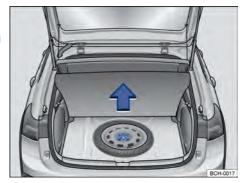
**Fig. 170** On the luggage compartment, under the floor lining: spare wheel and vehicle toolkit.
