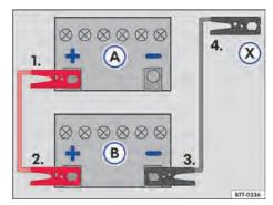
**Fig. 186** Jump lead attachment diagram: discharged vehicle battery (A) and battery in the vehicle providing assistance (B).
