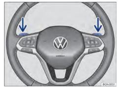
**Fig. 93** Steering wheel with Tiptronic gear shift paddles.
