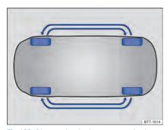
Fig. 198 Diagram showing how to swap wheels.
