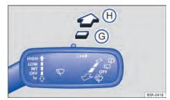
Fig. 73 To the right of the steering column: control the rear window wiper/washer.
