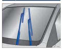
Fig. 173 Window wipers in service position.
