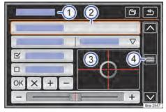
**Fig. 127** Schematic representation: overview of possible function buttons on the display.
