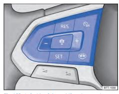
**Fig. 103** Left side of the multifunction steering wheel: ACC operating (variant 1) buttons.
