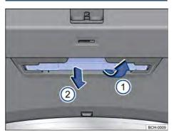
Fig. 46 On the rear lid: warning triangle holder.
