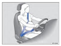
Fig. 30 Correct seat belt routing during pregnancy.
