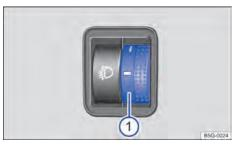
Fig. 71 Next to the steering wheel: control of the headlight range (1)
