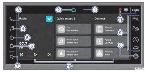
Fig. 153 Overview of controls (variant 1).
