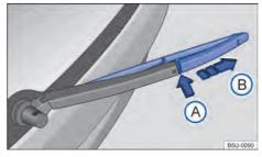
Fig. 175 Replacing the rear window wiper blades.
