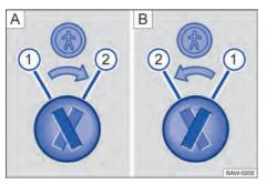
**Fig. 43** Childproof lock: A rear left door, B rear right door.
