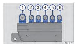
**Fig. 182** In the engine compartment on top of the battery: fuse arrangement.
