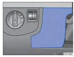
**Fig. 178** On the driver's side of the dashboard: fuse box cover.
