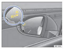
**Fig. 109** On the exterior mirrors: Blind Spot Monitor indicator.
