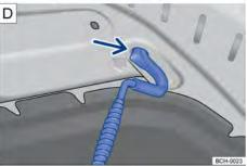
Fig. 188 © Bonnet stay. D Bonnet secured with the bonnet stay.
