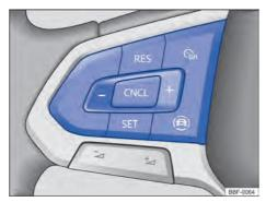
**Fig. 99** Left side of the multifunction steering wheel (version 2): speed limiter operating buttons.
