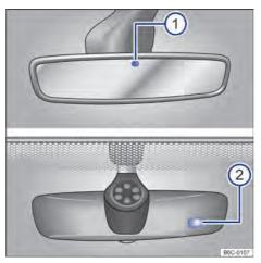
**Fig. 75** On the windscreen: automatic anti-dazzle interior mirror.
