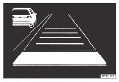
**Fig. 100** On the instrument cluster display: slower vehicle detected on the left-hand lane (schematic view).
