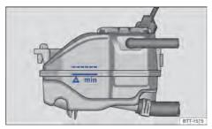
Fig. 193 On the engine compartment: marking on the coolant expansion tank.
