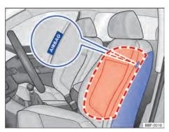
**Fig. 37** Front seat side: installation location and deployment zone of the side airbags.
