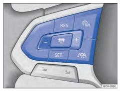
**Fig. 104** Left side of the multifunction steering wheel: ACC operating (variant 2) buttons.
