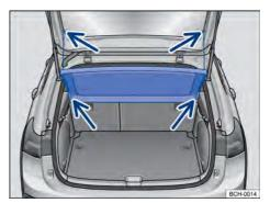
**Fig. 166** In the luggage compartment: remove and install the luggage compartment cover.
