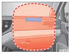
**Fig. 34** Installation location and expansion zone of the passenger front airbag.
