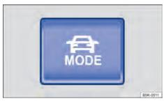
Fig. 95 On the top part of the centre console: MODE button to select driving mode.
