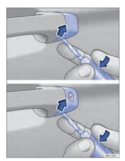
Fig. 53 Driver's door handle: remove cover.
