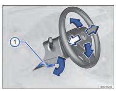
**Fig. 59** Below and to the left of the steering wheel next to the steering column trim: steering wheel position adjustment lever.
