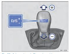
Fig. 92 Selector lever in Tiptronic position.
