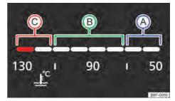
**Fig. 14** Engine coolant temperature indicator in the digital instrument cluster (version 2): (a) cold zone; (b) normal zone; (c) warning zone.
