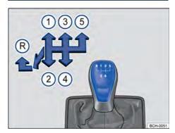
**Fig. 90** Gear shift pattern of a 5-speed manual gearbox.
