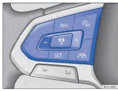
Fig. 108 Left-hand side of the multifunction steering wheel.
