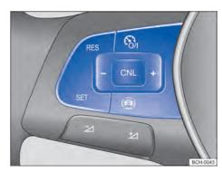
Fig. 98 Left side of the multifunction steering wheel (version 1): speed limiter operating buttons.
