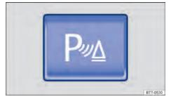
**Fig. 111** On the centre console or on the radio display again: button to enable and disable the park distance control (according to the vehicle version).
