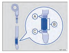
Fig. 191 Oil dipstick with markings.
