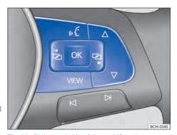
**Fig. 16** Right hand side of the multifunction steering wheel (version 1): menu operation and instrument cluster information exhibit buttons.
