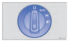
**Fig. 69** Next to the steering wheel: light switch (one variant).
