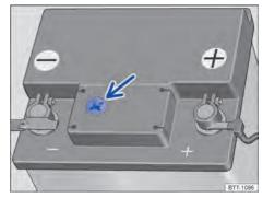
**Fig. 196** On the engine compartment: example of display position on the upper side of the vehicle battery.
