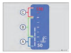
**Fig. 13** Engine coolant temperature display on the digital instrument cluster: (a) cold zone; (b) normal zone; (c) warning zone.
