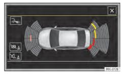
**Fig. 112** Indication on the radio system: full screen mode. The detected areas depend on the vehicle version
