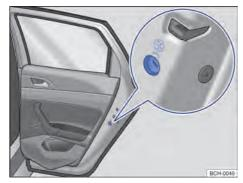
Fig. 44 On the rear door (right-hand side): child-proof lock.
