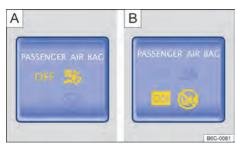
Fig. 32 In the upper part of the centre console: front passenger front airbag indicator lamp off A or on B.
