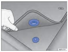
Fig. 18 Driver side mat attached to the floor pin.
