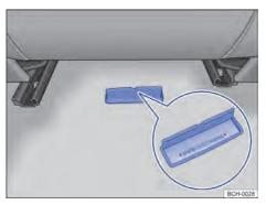
**Fig. 211** In front of the rear passenger seat, on the right-hand side of the floor: vehicle identification number (running gear number).
