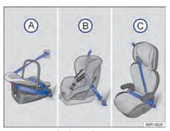
Fig. 39 Figures (A), (B) and (C) illustrate the main securing points for the child restraint system for children only wearing the seat belt.
