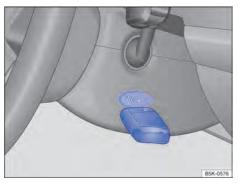
**Fig. 88** To the right of the steering column: emergency start function of vehicles with Keyless Access locking and start system.
