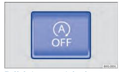
**Fig. 89** On the centre console: Start-Stop system button (depending on vehicle version).
