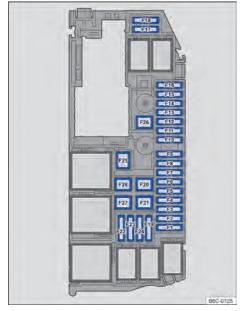
**Fig. 181** In the engine compartment: fuse arrangement.
