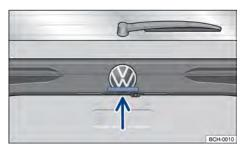
Fig. 56 On the boot lid: button to open the boot lid.
