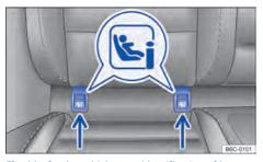
**Fig. 41** On the vehicle seat: identification of lower retaining rings for child seats.
