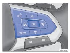
**Fig. 17** Right hand side of the multifunction steering wheel (version 2): menu operation and instrument cluster information exhibit buttons.
