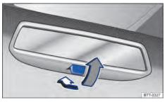
**Fig. 76** On the windscreen: manual anti-dazzle interior mirror.
